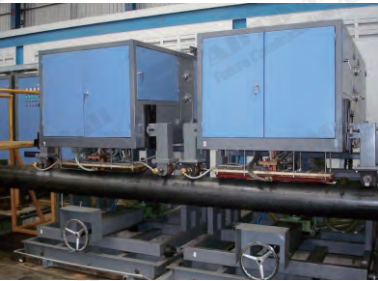
8.On-Line Weld Seam Annealing
