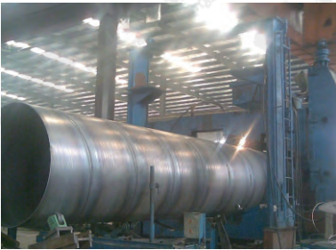
7.Spiral Submerged Arc Welding
