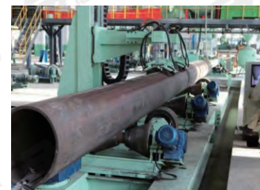
4. Longitudinal Submerged Arc Welding
